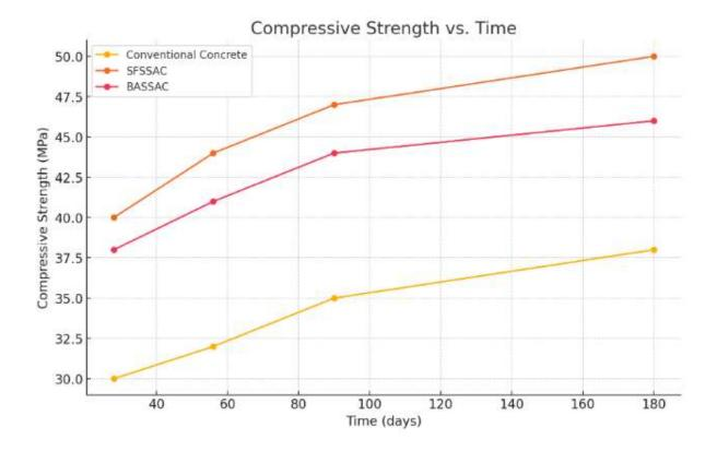
Compressive Strength vs. Time: This line graph shows the increase in compressive strength over time for conventional concrete, SFSSAC, and BASSAC mixes.
