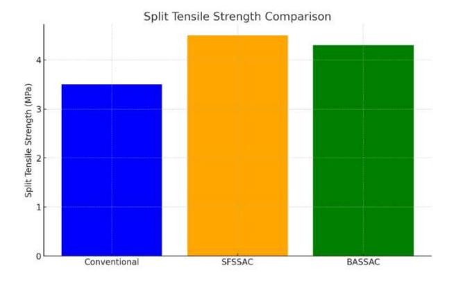
Split Tensile Strength Comparison: A bar chart comparing the split tensile strengths of conventional concrete, SFSSAC, and BASSAC mixes.
